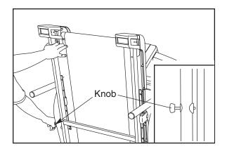
Hold the metal frame firmly with both hands, and lower the treadmill to the floor. CAUTION: To decrease the possibility of injury, do not lower the treadmill by gripping only the plastic foot rails. Do not drop the treadmill frame to the floor. Be sure to bend your legs and keep your back straight.
